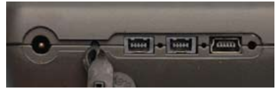
The remaining connectors lie along the top edge, above the screen. On the left is the DC power/charger input, with the COM, USB and HOST sockets alongside (left to right).
