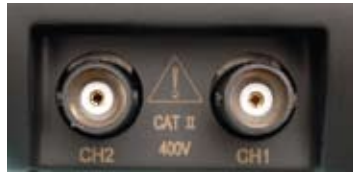
The two scope inputs are on the lower right side of the meter, adjacent to the multimeter inputs.
